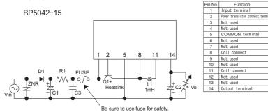
For acutual usage, Please kindly evaluate and confirm our part mounted in your product, Especially, Please make sure to confirm the load current does not exceed Max. rated current by using the current probe.
